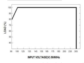
X De-rating is needed under low input voltage.
