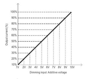
Applying additive 10V PWM signal(frequency rang 100Hz-3KHz)
