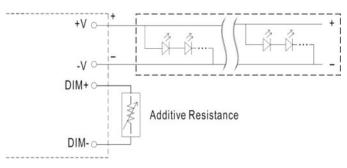
DO NOT connect "DIM- to V-"
