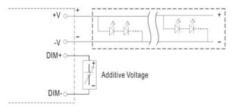
DO NOT connect "DIM- to V-"
