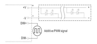
DO NOT connect "DIM- to V-"
